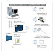
Distech Controls offers wireless communication on an open platform. Our controllers are enabled with wireless receivers, delivering room information to the network via LONWORKS® and your choice of platform: flat LonWorks or EC-Net powered by the Niagara<sup>AX</sup> Framework<sup>TM</sup> for web-based, LonWorks and BACnet® compatibility.
