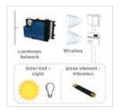
Our wireless battery-less devices are powered by different kinds of ambient energy - energy harvesting technology - such as light and vibration. Energy harvesting provides ecological compatibility, eliminating batteries and the use of cable material (copper, plastics etc.). Energy harvesting also allows for an important quality improvement, making these devices virtually service-free.
